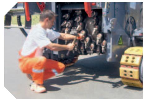
Readily accessible milling drum to allow tool replacement in no time at all
