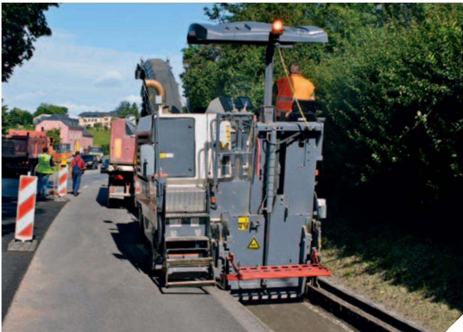
Using FCS to cut narrow trenches and channels ▼
