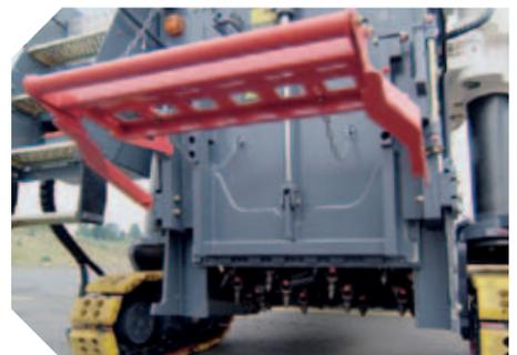
▲ Hydraulically adjustable side plates close the milling chamber on the right ...
