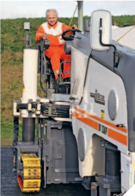
▲ Full control from the driver's seat, which can be moved out over the side of the machine
