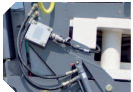
Wire-rope sensor for highly precise milling depth control
