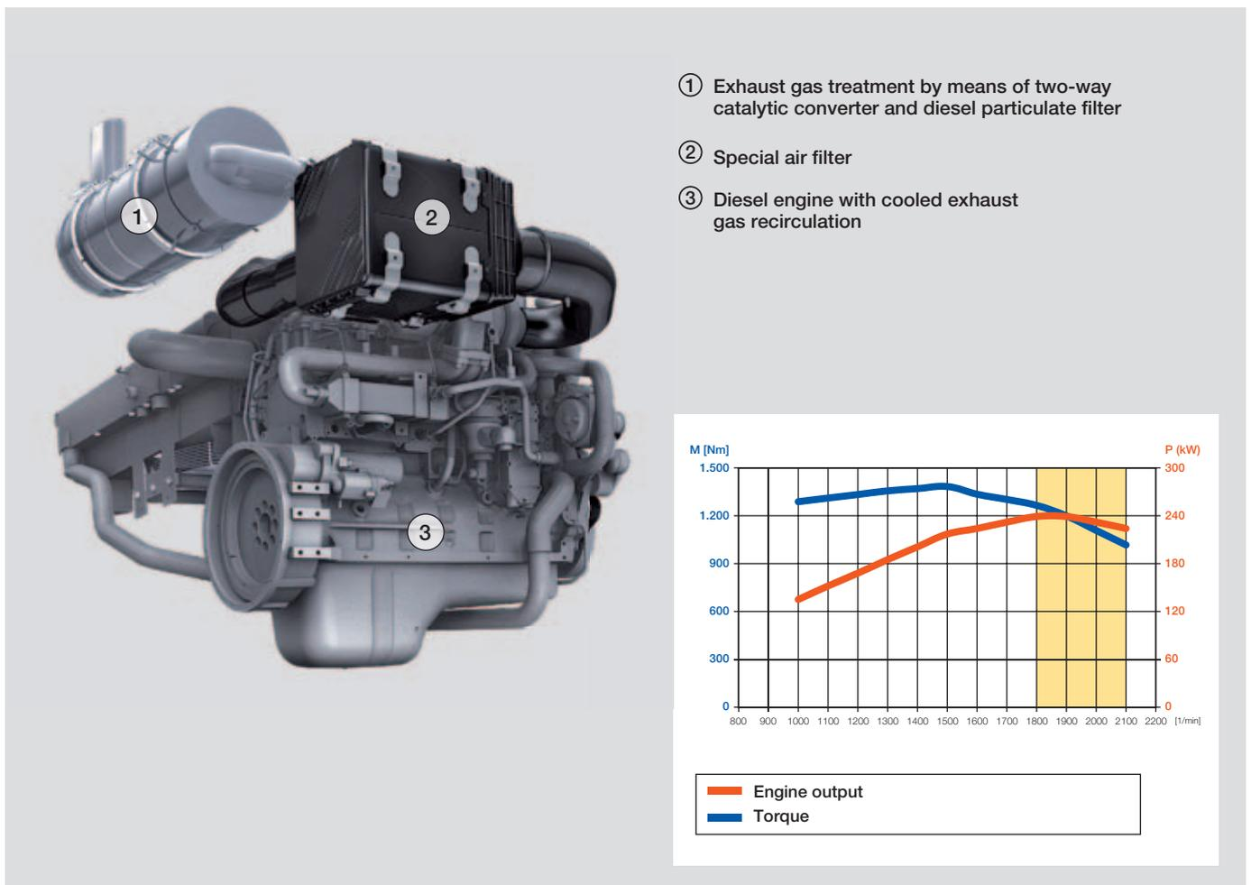
▶ The W 100 Fi, W 120 Fi, W 130 Fi features state-of-the-art engine technology for lowest environmental emission levels, complying with the stringent specifications of exhaust emission standards EC Stage 3b / US Tier 4i.
